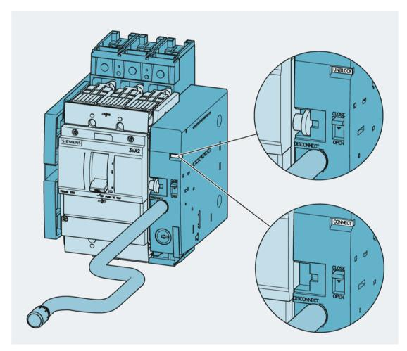
In the draw-out version, the 3VA molded case circuit breaker is supported by the side walls of the draw-out unit and can be moved into three defined positions by rotation of a crank handle. The current breaker position is indicated by the position indicator.
