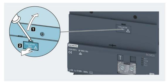
Disconnection of the main conductor connections is thus unnecessary. On completion of the tests, the circuit breaker must be pushed back into position before the residual current device is commissioned.
