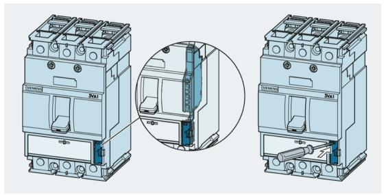
The trip must be reset by deliberate acknowledgement of the fault before the molded case circuit breaker is switched to ON again.
