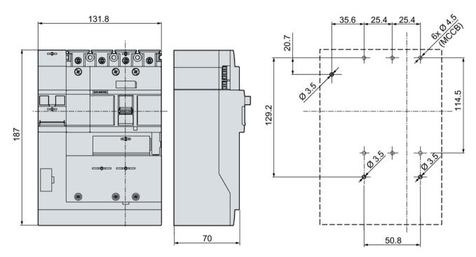
With 4-pole 3VA1 molded case circuit breaker size 160 A
