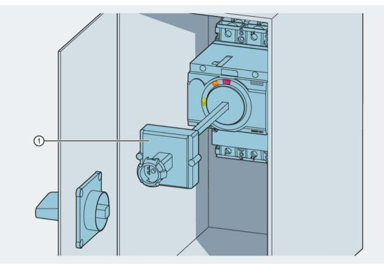
① Tolerance compensator
