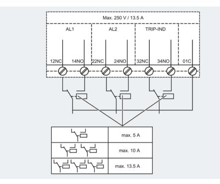
The terminal designations of the relevant contact, the maximum rated voltage and the current carrying capacity are shown in the diagram below.
