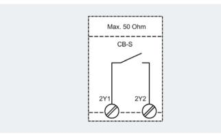
When the molded case circuit breaker is reset and then switched on again, the contacts .1C and .2NC of the auxiliary switch are closed and the tripped display on the residual current device is reset.
