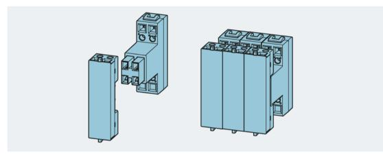
The breaker-end half is attached to the underside of the molded case circuit breaker and electrically connected to the internal accessories. Appropriate openings and cable ducts are provided in the molded case circuit breaker for routing stranded wires. The plug-in socket half of the auxiliary circuit connector is inserted in the socket and electrically connected to the customer's installation.
