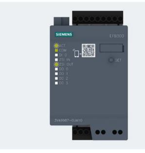
In order to select the next output, press the <SET> button briefly ①. The LED of the next output starts to flash ②, the output is selected.
