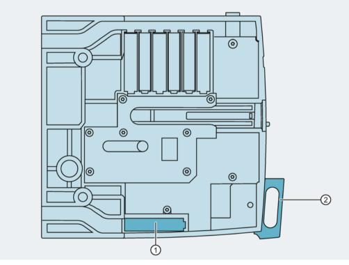
① Slot for position signaling switch for signal "Draw-out unit locked / open"
