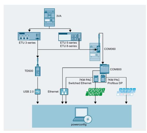
The possible means of connection of the COM800 / COM100 breaker data server are described in detail in the 3VA Communication system manual (see Reference documents (Page 12)).
