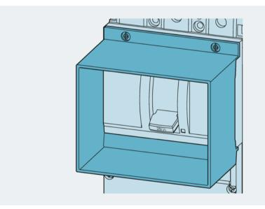
The door cutout must be positioned such that it is flush with the door feedthrough. It must also be positioned in such a way as to minimize the size of the gap between the feedthrough walls and the cutout. An escutcheon can be fitted as well in order to obtain an optimum finish.
