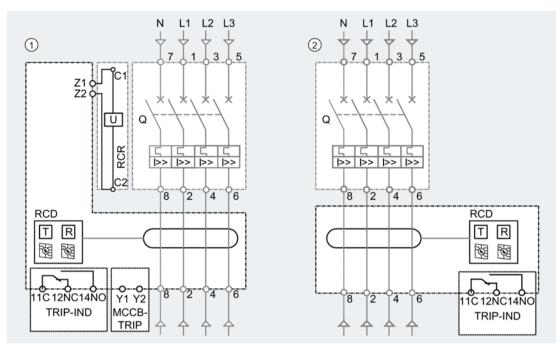
Side mounted RCD basic, 3-pole and 4-pole
