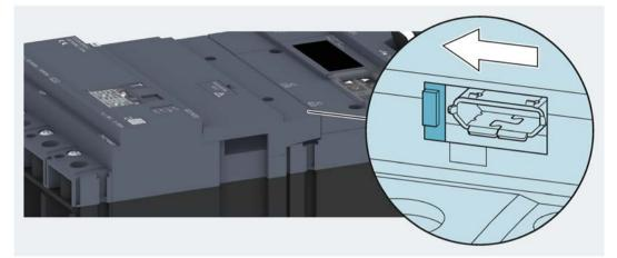
3. Insert one end of the connecting cable into the interface on the residual current device. The interfaces and the connecting cable are labeled to ensure that the cable ends are inserted in the right interfaces.
