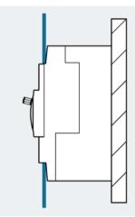
Handle and release are freely accessible, the control cabinet door closes flush with the molded case circuit breaker.
