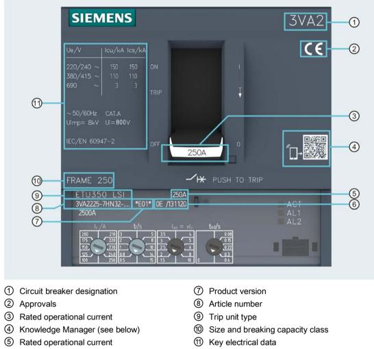
The following information is displayed on the front panel of the circuit breaker:
