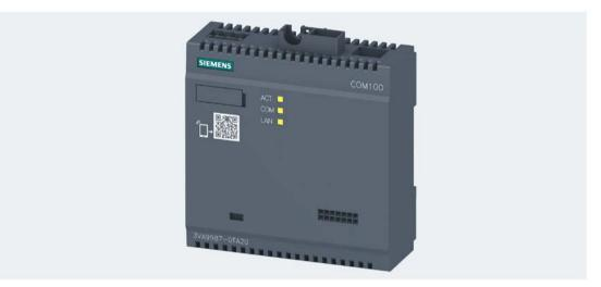
The COM100 is identical in design to the COM800 breaker data server, i.e. it is connected directly to the COM060 communication module in the 3VA2 molded case circuit breaker by means of a cable. By contrast with the flexibility offered by the COM800 breaker data server, only one single 3VA2 molded case circuit breaker can be connected to each COM100 unit.
