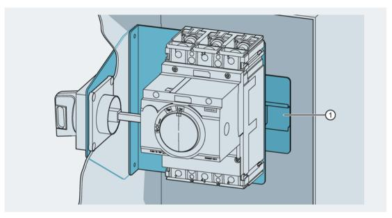
If there is insufficient space available on the mounting plate to install terminals, a terminal plate 1 can be bolted to the cubicle.
