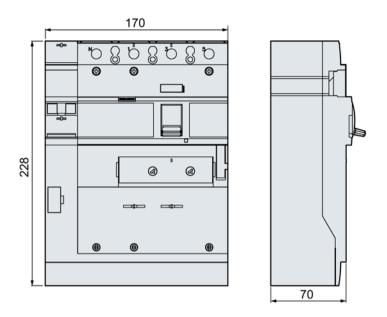
With 4-pole 3VA1 molded case circuit breaker size 250 A (Basic RCD510 only)
