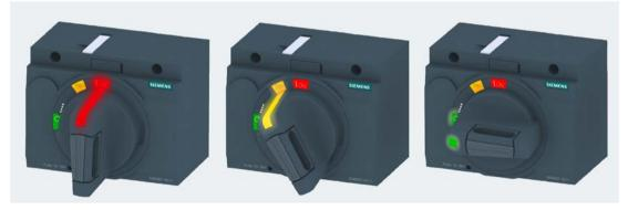
You can retrofit an active illumination kit to manual rotary operators. The illuminated indicator in the rotary handle signals the relevant switching position in the colors red, yellow and green. This provides clear visualization of the switching position on-site in conditions of poor visibility. 2.2 Ergonomic design
