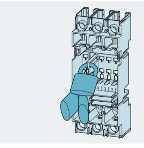
The socket unit can be locked by padlocks to prevent the insertion of a 3VA molded case circuit breaker while maintenance or overhaul work is in progress. Using these locks to prevent insertion and operation of a molded case circuit breaker helps to protect personnel and the installation itself. The socket unit of the plug-in socket is equipped with three openings for padlocks.
