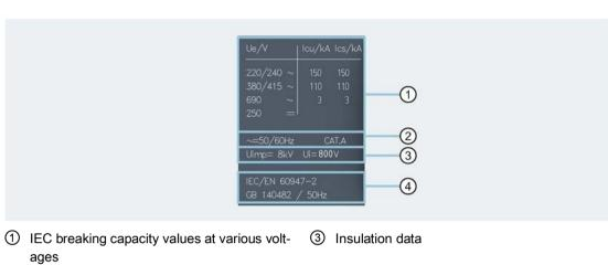
The key electrical data label on the molded case circuit breaker displays the following information:
