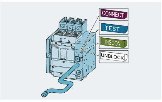
The switching position is indicated in a window of the draw-out unit and is clearly colorcoded, enabling immediate identification of the current switching position of the molded case circuit breaker.
