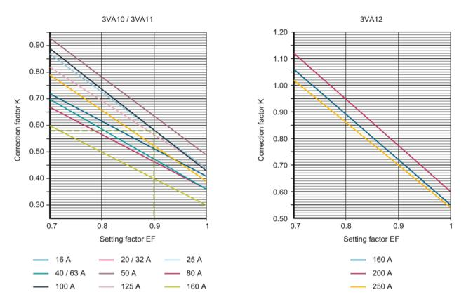
Using the setting factor calculated at 50 °C, it is possible to read the correction factor K off the following charts:
