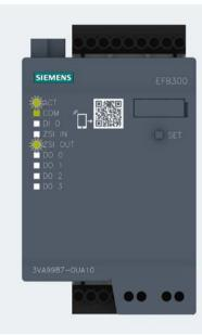
3. In order to activate the selected output, press the <SET> button for longer than 2 seconds.
