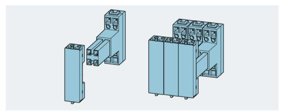
The breaker-end half is attached to the underside of the molded case circuit breaker and electrically connected to the internal accessories. Appropriate openings and cable ducts are provided in the 3VA molded case circuit breaker for routing stranded wires. The socket-end half of the auxiliary circuit connector with the movable telescopic rail is inserted in the socket and electrically connected to the customer's installation.
