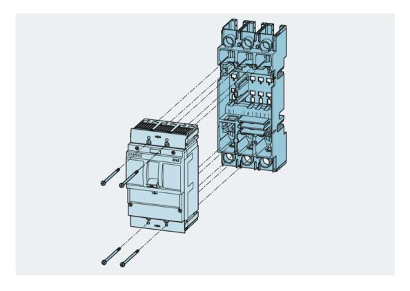
With a plug-in system, the molded case circuit breaker is moved into and out of the plug-in socket manually.
