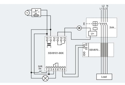
The circuit diagram below shows a typical MRCD circuit with an undervoltage release.
