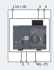
Motor operator actuation controlled via control cable
