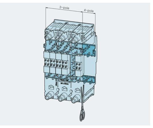
Cable cages consist of a top half and a bottom half. These parts are designed such that they cannot be mounted in the wrong position at the rear of the molded case circuit breaker.
